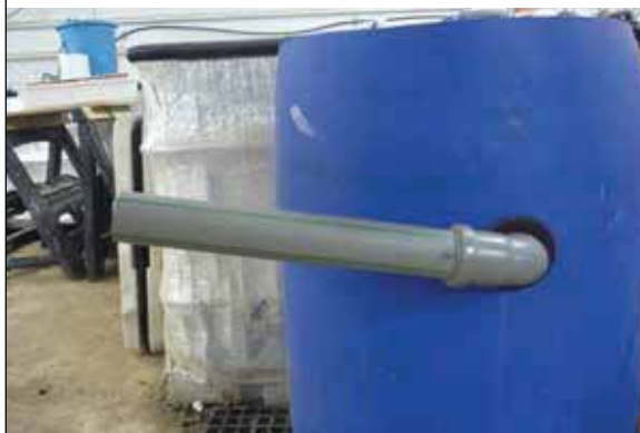
FIGURE 9.13 Overflow pipe on a biofilter
