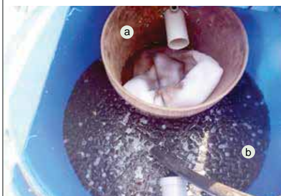
FIGURE 4.30 Details of biofilter showing the (a) additional mechanical filtration and (b) the biofilter medium
