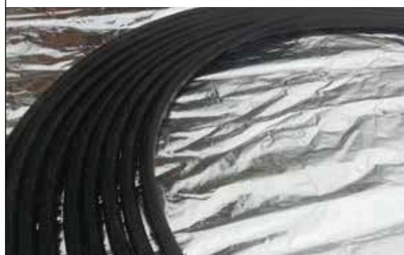
FIGURE 9.11 Water heating technique using black tube arranged in a spiral
