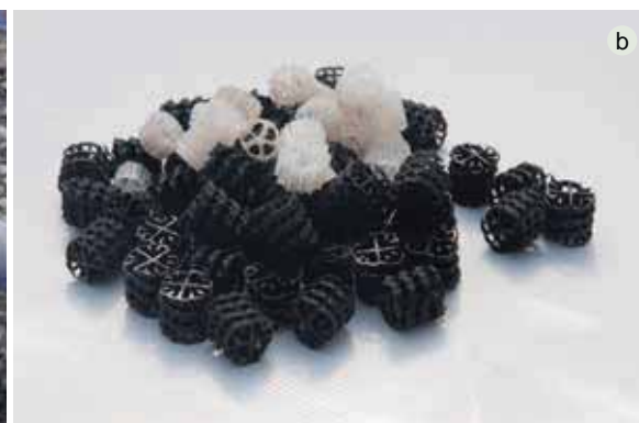
FIGURE 2.9 Aerated biofilter (a) containing plastic filter medium (b)
