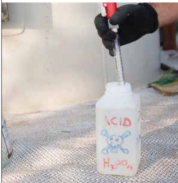
FIGURE 3.11 Phosphoric acid ( \text{H}_3\text{PO}_4 – 85% concentration) used to lower pH
