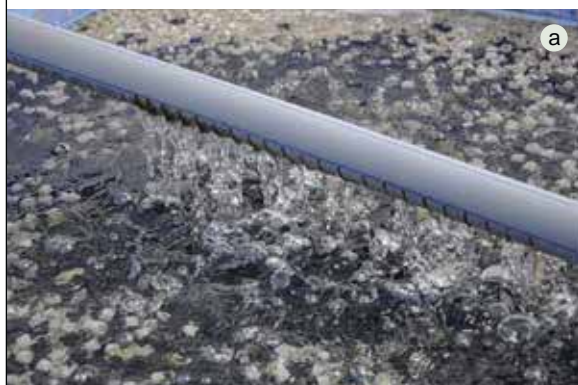
FIGURE 2.9 Aerated biofilter (a) containing plastic filter medium (b)
