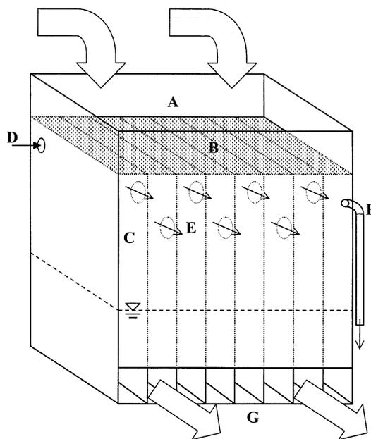
Fig. 1. Typical LHO configuration and components showing water flowing into a collection trough or plate (A), through a perforated distribution plate (B), and is oxygenated in the chambers (C), as gas flows from inlet gas port (D), through holes between chamber to chamber (E), to the off gas port (F), where excess gas is bubbled off under water. Water exits at the bottom of the unit (G).
