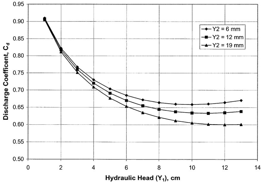
Fig. 2. Discharge coefficient,  $C_d$ , as affected by hole diameter ( $Y_2$ ) and hydraulic head ( $Y_1$ ).
