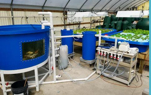
**Demonstration of a** Small Scale **De-coupled Aquaponics System** Utilizing Floating Bead **Bioclarifier and Airlift** Technology
